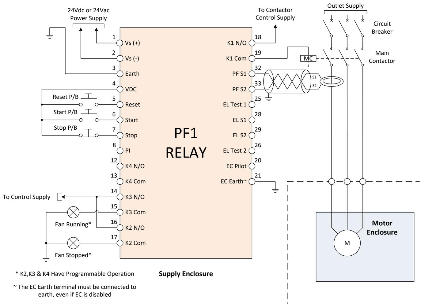
Figure 3.2: Typical Application - Fan Protection (Only)
