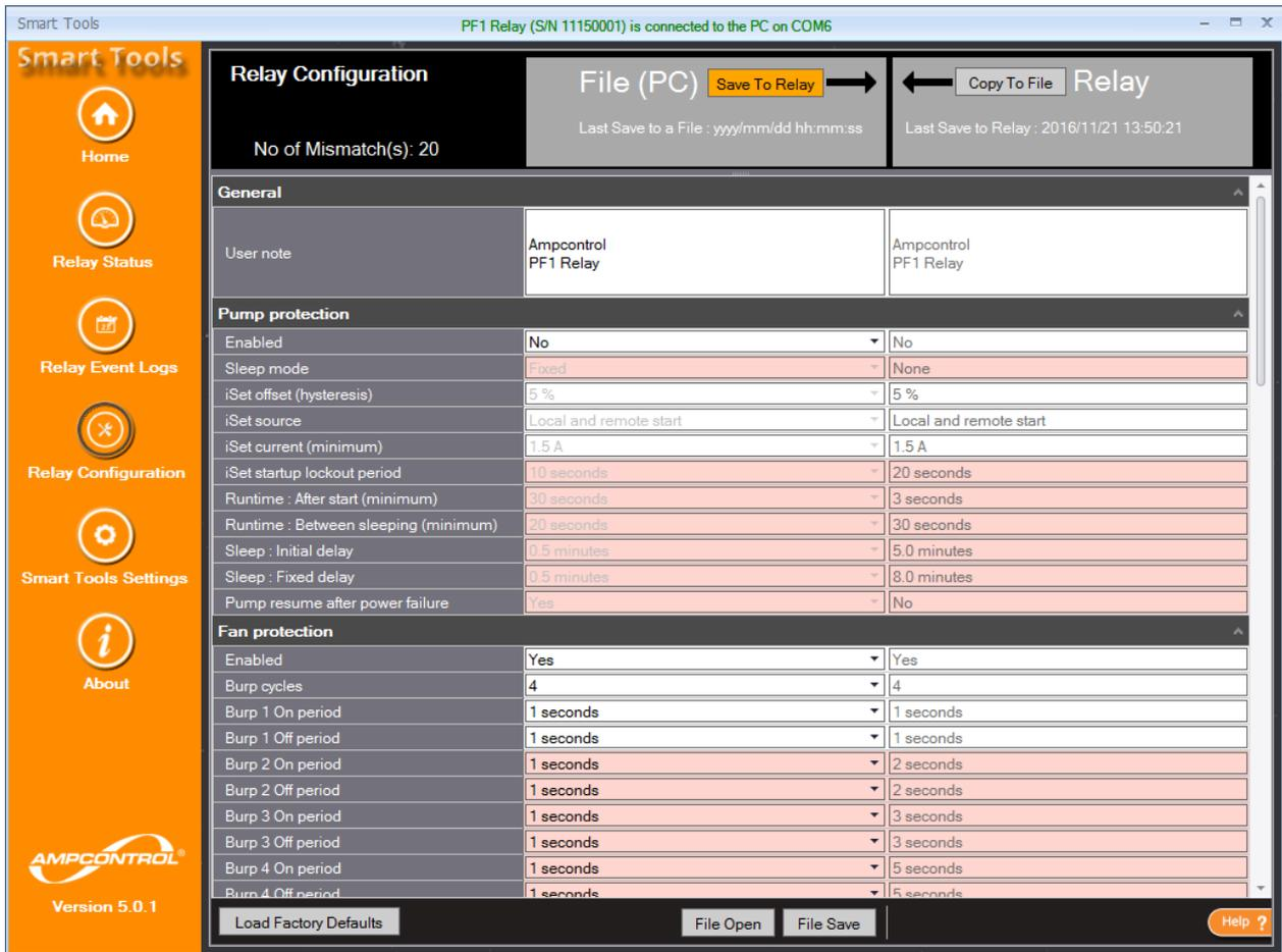
Figure 10.4: Smart Tools Software - Relay Configuration Page
