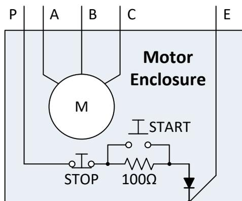
Figure 9.1: Remote Start & Remote Stop Implementation
