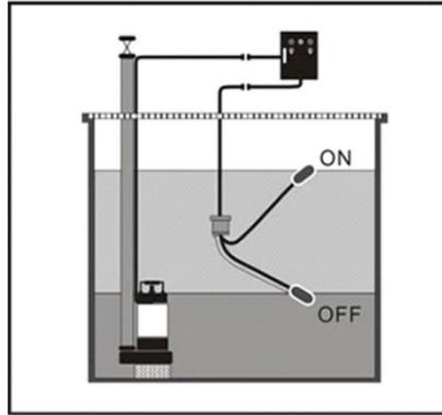
Figure 6.5: Pump Float Switch
