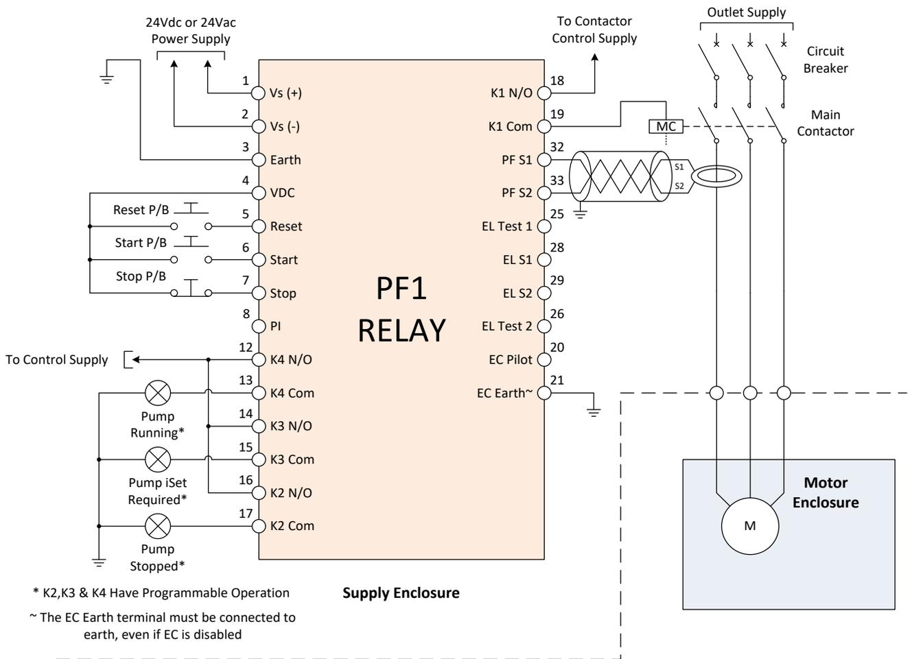
Figure 3.1: Typical Application - Pump Protection (Only)
