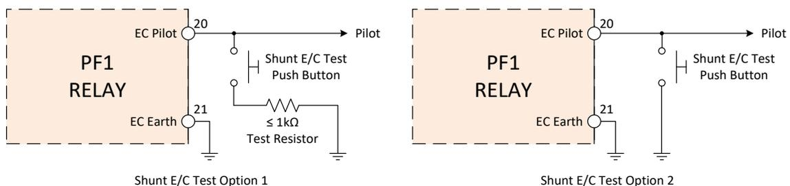
Figure 5.3: Earth Continuity Shunt Test Wiring Options
