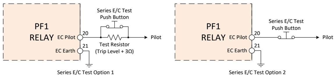
Figure 5.2: Earth Continuity Series Test Wiring Options
